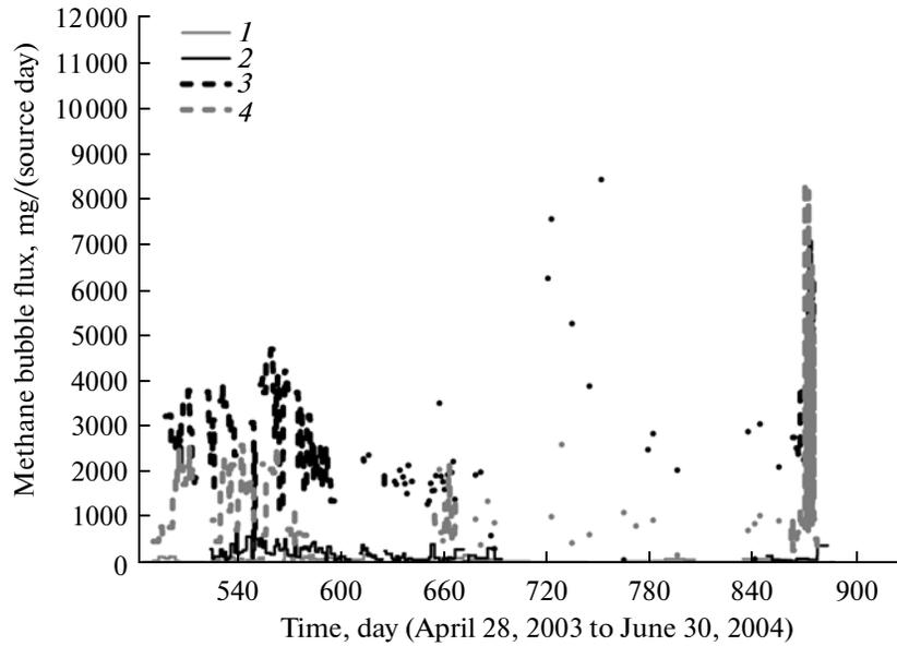
**Fig. 2.** Point-source and hotspot methane bubble fluxes in four parts of Shuchi Lake (northeastern Siberia) from measurements [11] (April 28, 2003, to June 30, 2004). (1) Thermokarst margin in a deep-water part (depth 7.4 m), point source; (2) thermokarst margin in a shallow-water part (depth 1.75 m), point source; (3) thermokarst (depth 2.25 m), hotspot; and (4) thermokarst in deep water (depth 4.75 m), hotspot.
